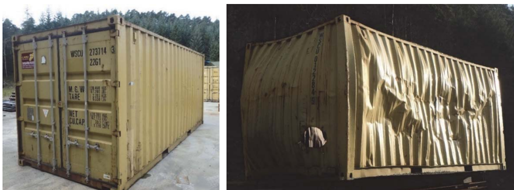
Figure 2: A 20-foot container before (left) and after (right) testing.
