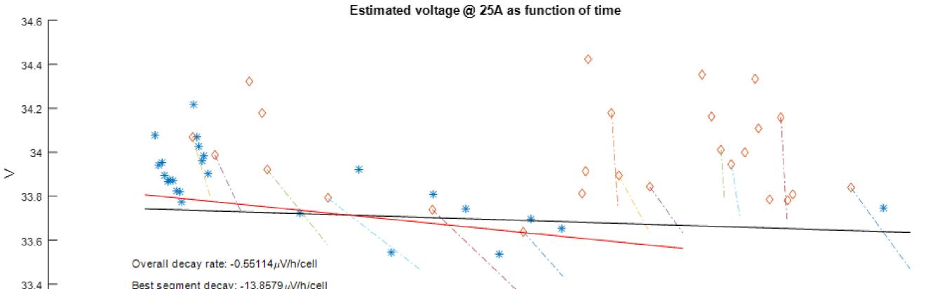
After the data logs were analysed, it was found that both systems exhibited very low degradation rates: compared to Dantherm Power's nominal rate of  $2 \mu V/h$ , system #2 had a tenfold improvement:  $0.2 \mu V/h$ . System #1 even showed a marked voltage rejuvenation,  $-4 \mu V/h$ .
