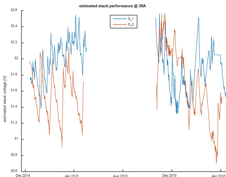
Figure 1: Stack performances through the two test campaigns.
