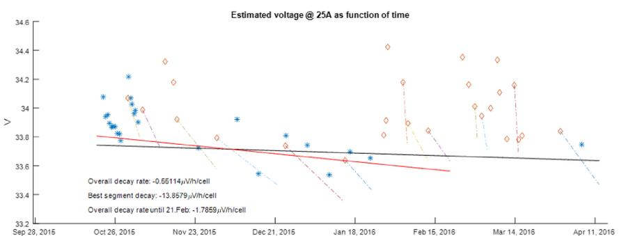
Figure 2: System **#1**'s performance in the second campaign. Every diamond  $\diamond$  is a start-up, followed by a dashed line of continuous operation. Every asterisk  $*$  is a measurement on a polarisation curve.
