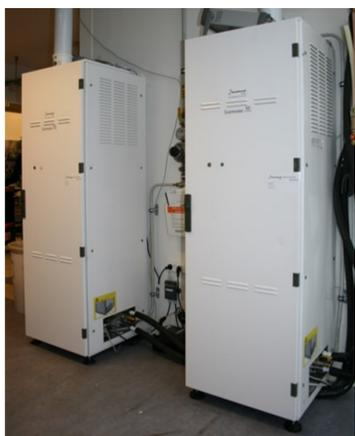
The SAPHIRE consortium planned a test campaign on  $\mu$ CHP PEMFC systems, which was executed by partner Dantherm Power (today Ballard Power Systems Europe). The objective of the experimental campaign was to test two  $\mu$ CHP systems in nominal conditions for **3000 hours** of operation each, to provide a baseline for system degradation. Two stacks that had already been operated in a field trial for 5000 hours were selected to remove break-in effects.
