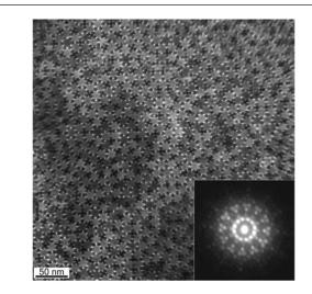
**Figure 5.** A dodecagonal quasicrystalline superlattice selfassembled from 13.4 nm  $Fe_2O_3$  and 5 nm Au nanocrystals. Inset shows a selected area electron diffraction pattern with crystallographically forbidden 12-fold rotational symmetry. Adapted from Reference 30.
