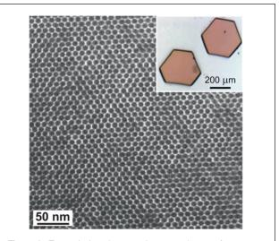
Figure 3. Transmission electron microscopy image of a superlattice self-assembled from 7.5 nm PbS nanocrystals. The inset shows optical micrographs of three-dimensional "supercrystals" grown from nanocrystals.<sup>19</sup>
