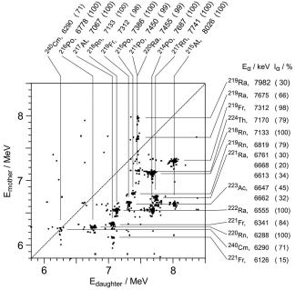
Fig. 6. Energies of mother-daughter delayed coincidences of events during the beam pauses within time and position windows of 1s and  $\pm 1$  mm, respectively. Given literature values of  $\alpha$  energies and intensities were taken from [64]. The spectrum includes data measured during 25 days beginning May 5. Strip numbers 5, 9, 13 and 15 are not included, see text for details.
