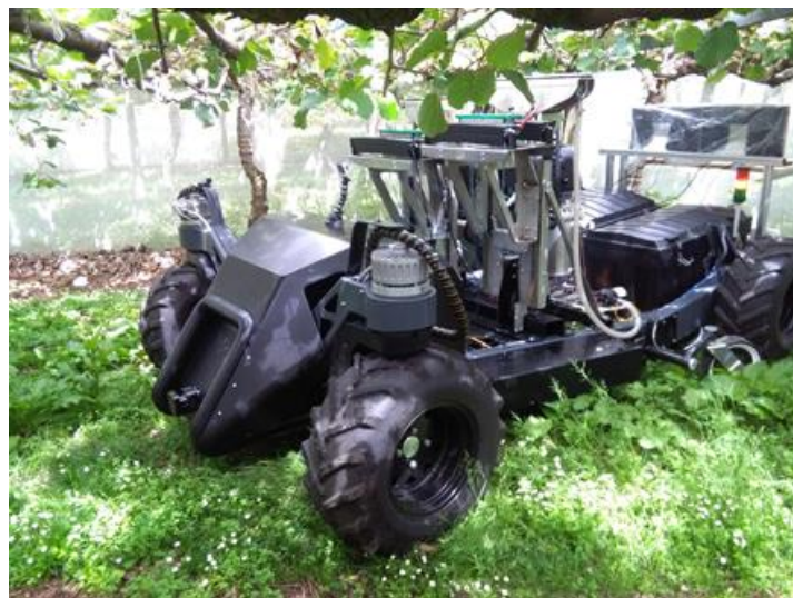
Figure 6. Pollination system mounted on the platform (in orchard)
