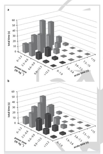
**Fig. 1** Exposure variation analysis of the penultimate  $5 \min \mathbf{a}$ , and last  $5 \min \mathbf{b}$  of competition prior to the sprint. Black columns represent the time spent in short-duration and high-intensity efforts (i. e., >6.6 W · kg<sup>-1</sup> and <3.8 s).
