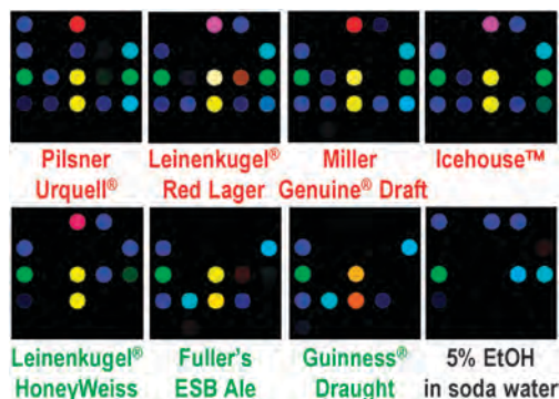
Fig. 45 Colorimetric array analysis of a complex mixture: headspace analysis of various beers compared to 5% ethanol in carbonated water. Brands in red are lagers, brands in green are ales. Reproduced with permission from ref. 10.
