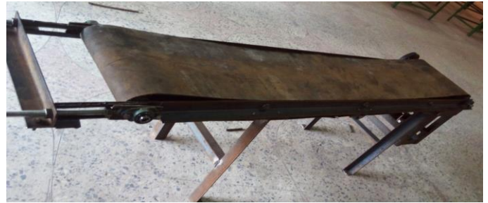
Figure 1: The Developed Belt Conveyor
