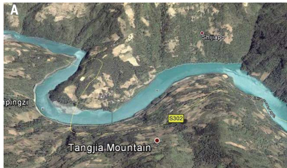
Fig. 1. Geographical configuration of dammed lakes and flow attenuation equation. (A) Vicinity of the Tangjiashan dammed lake. Landslide dam formation is subject to river topology and other random factors and therefore can hardly be of uniform height across the river. A
