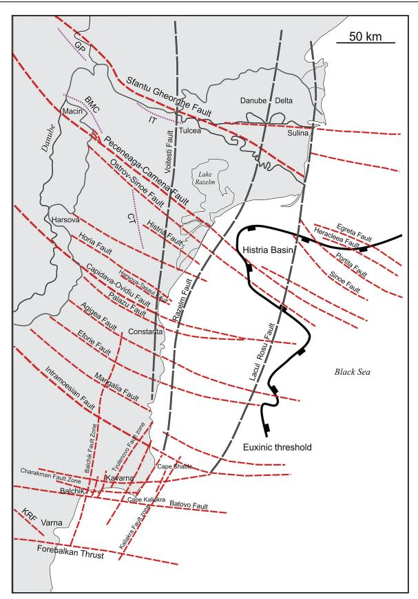
Fig. 2. Major faults on the north-western Black Sea margin. Purple dotted lines are lineaments of seismic instability. Abbreviations: KRF, Kemanlar-Ruslar Fault; GP, Galați-Pechea line; IT, Issacea-Tulcea line; CT, Cogealac-Topolog line; BMC, Brăila-Măcin-Cerna line.
