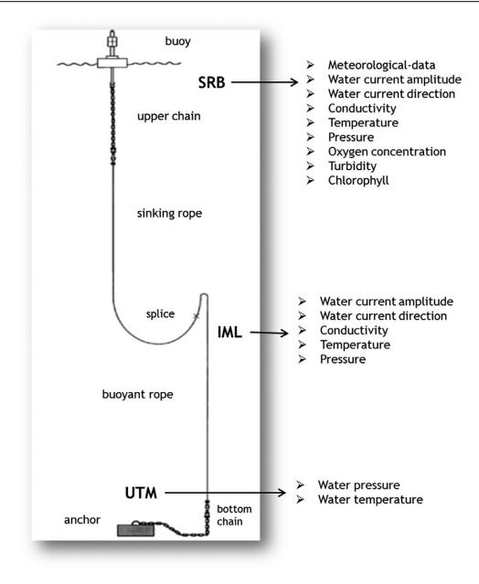
Fig. 6. Types of data collected from the EUXINUS buoys. Abbreviations: SRB, surface relay buoy; IML, intermediate module layer; UTM, underwater tsunamometer module.
