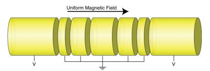
Figure 1. Example of a Penning-Malmberg trap similar to those used in the antihydrogen experiments. Particles are confined radially by a strong uniform axial magnetic field. Axially they are confined by the electric fields generated by biasing the conducting, but individually insulated cylinders (called electrodes). In practice, more electrodes are needed for antiparticle manipulations and the ALPHA, ATHENA and ATRAP experiments use up to fifty individually controllable electrodes.
