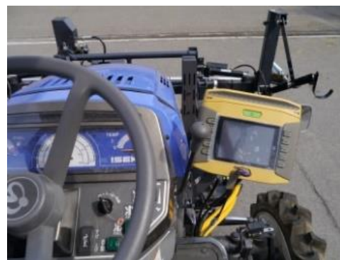
Figure 4. Smart 2nd fertilizer application system with CropSpec. The height of sensor is 3m and the length of fertilizer distributor is 15m
