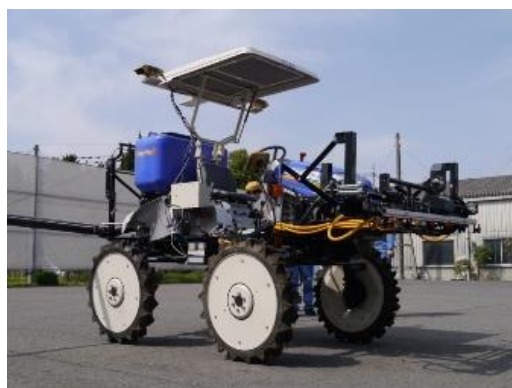
Figure 4. Smart 2nd fertilizer application system with CropSpec. The height of sensor is 3m and the length of fertilizer distributor is 15m
