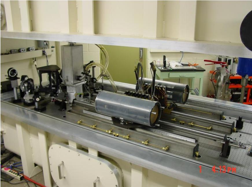
2-m FTS. Wavelength range 300 nm – 5.5  $\mu\text{m}$ .
