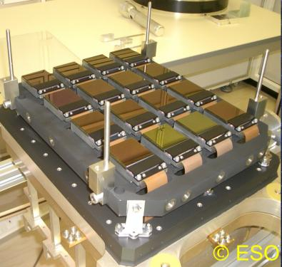
VISTA: 4m, fov: 1.65° Ø, px: 0.34" VIRCAM: ZYJHKs+NB 16x2048<sup>2</sup> Raytheon dets
