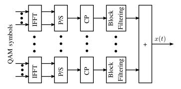
Fig. 1. F-OFDM block diagram.
