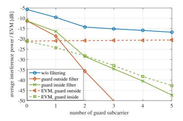
Fig. 6. Interference to neighboring subband versus number of guard subcarrier
