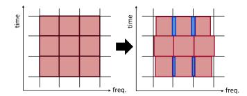
Fig. 3. Guard bands keeping regular resource grid.
