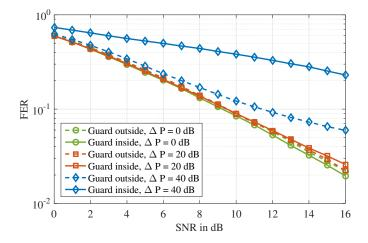
Fig. 10. FER performance for F-OFDM with different number of guard subcarriers, EPA channel, 3 km/h, QPSK,  $R_c = 0.32$ , 2 guard SCs.
