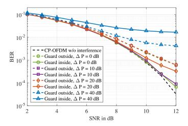
Fig. 8. Uncoded BER performance of F-OFDM on an AWGN channel with 2 guard SCs and QPSK modulation.
