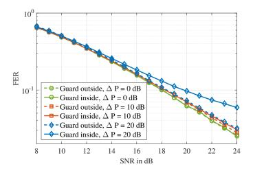
Fig. 11. FER performance for F-OFDM with different number of guard subcarriers, EPA channel, 3 km/h, 16-QAM,  $R_c = 0.55$ , 2 guard SCs.
