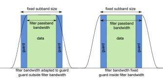
Fig. 4. Two approaches to keep regular resource grid.
