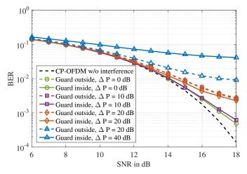
Fig. 9. Uncoded BER performance of F-OFDM on an AWGN channel with 2 guard SCs and 16QAM modulation.
