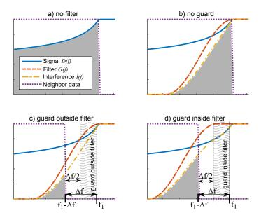
Fig. 5. Guard bands keeping regular resource grid
