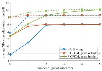
Fig. 7. SINR of edge subcarriers versus number of guard subcarrier for SNR=10 dB, outmost SC (solid) and second outmost SC (dashed)
