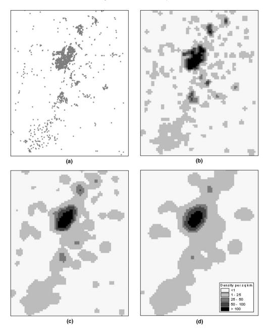
Fig. 1. Kernel density mapping: (a) distribution of point event data, (b) 250 m grid, 500 m bandwidth, (c) 250 m grid, 1000 m bandwidth, (d) 250 m grid, 1500 m bandwidth.
