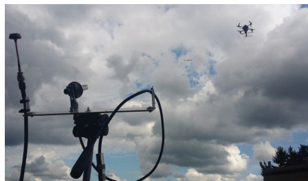
Figure 8. ICARUS COM tools communicating with aerial robotic systems (acting as communication relays). (Source: ICARUS).
