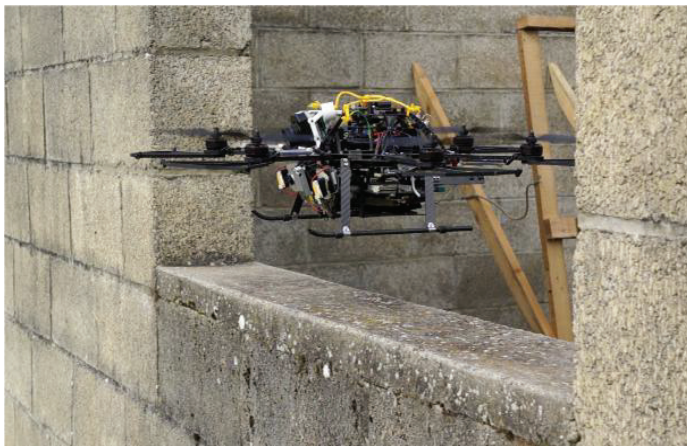
Figure 11. Skybotix multicopter flying through a window for inspecting a building from the inside (source: ICARUS consortium).
