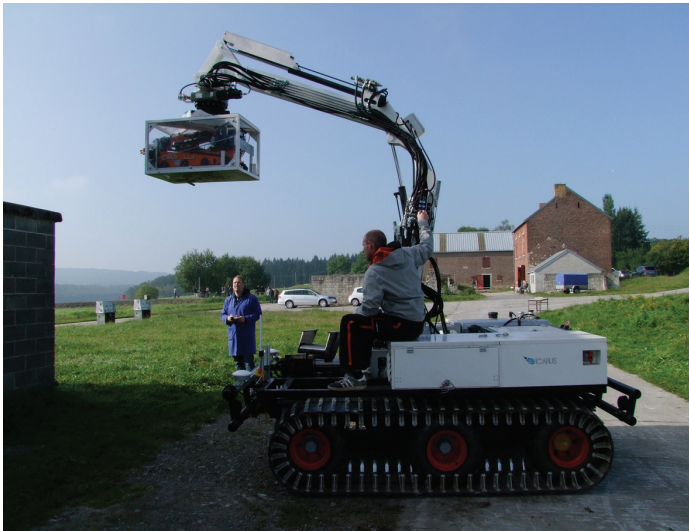
Figure 13. The LUGV uses its arm to lift the transport box containing the SUGV (Source: ICARUS).
