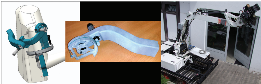
Figure 29. (i) SAM exoskeleton upper part advanced design and rapid prototyping part integration test. (ii) LUGV with extended manipulator (source: ICARUS).
