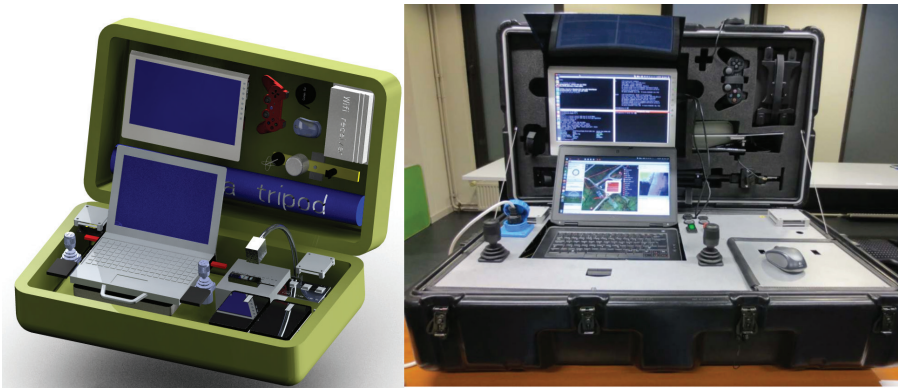
Figure 28. Portable RC2 CAD model (left) and finished RC2 rugged system (right) (source: ICARUS).
