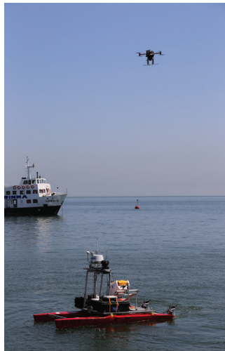
Figure 6. Rotary wing unmanned aircraft providing victim's location to ROAZ II (source: ICARUS).
