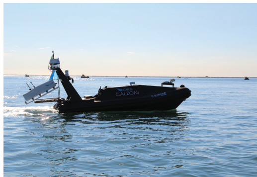
Figure 13. ICARUS unmanned surface vehicle deploying the unmanned rescue capsule (source: ICARUS).
