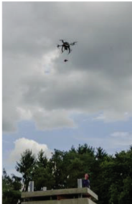
Figure 10. Eurecat quadrotor delivering a first aid kit to an injured victim (source: ICARUS consortium).
