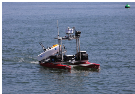
Figure 8. Unmanned capsule being launched from ROAZ II (source: ICARUS).
