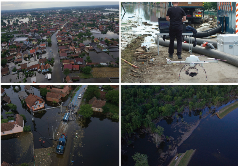
Figure 28. Top left: Flooded city of Orasje; top right: UAV used for the operations; bottom left: optimization of the location for the B-FAST water pumps and bottom right: broken dam on the Sava river detected by the UAV (source: ICARUS).
