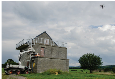
Figure 24. Large UGV deploying small UGV on the first floor, assisted by the outdoor rotorcraft (source: ICARUS).
