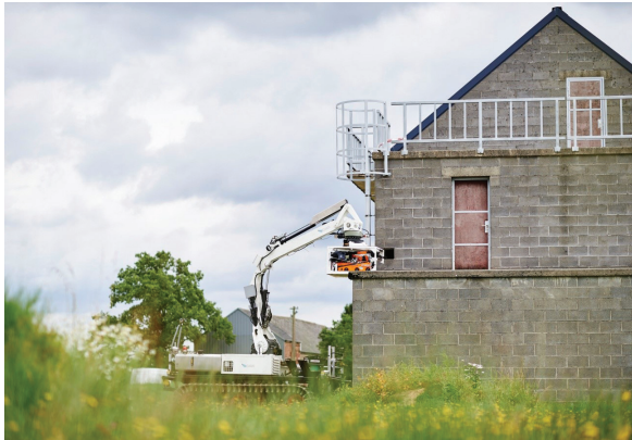
Figure 12. ICARUS large unmanned ground vehicle deploying the small unmanned ground vehicle on the top of a building (source: ICARUS).
