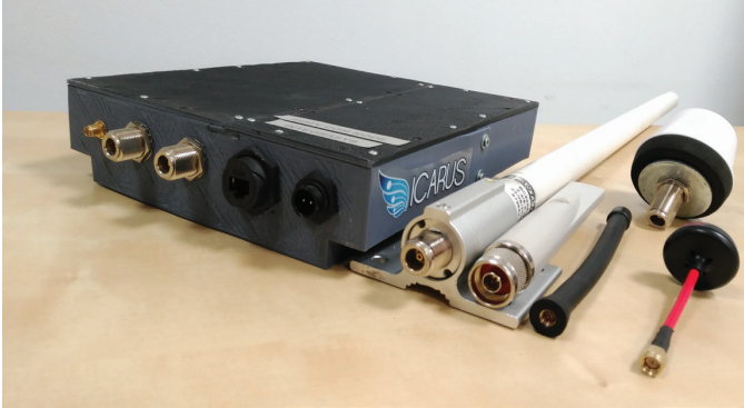
Figure 4. SUGV COM box and set of antennas used in various missions. (Source: ICARUS).
