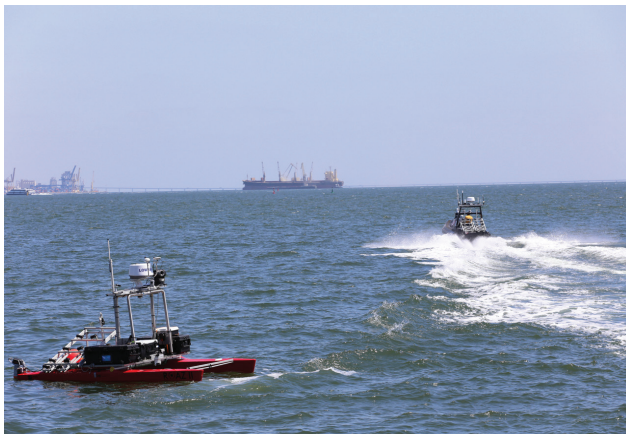
Figure 10. U-RANGER and ROAZ II providing situational awareness to rescue workers behind the ferryboat (source: ICARUS).
