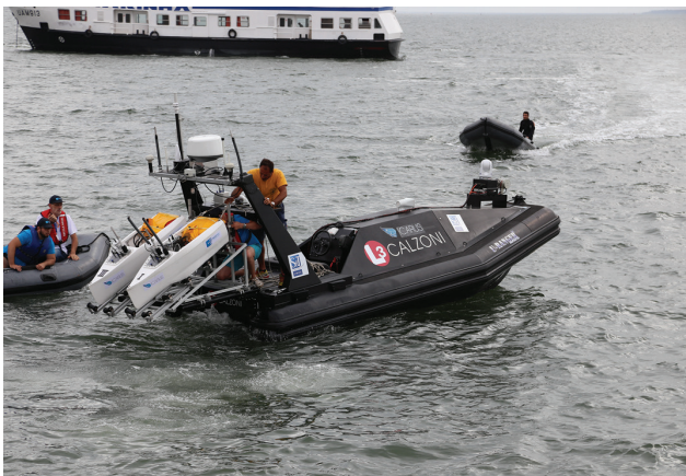
Figure 13. Two UCAPs mounted on the deployment system installed on the U-RANGER (source: ICARUS).
