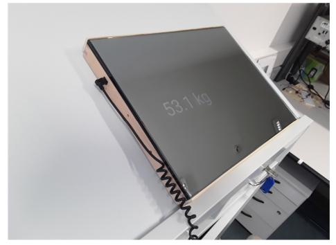
Figure 19: Smart Mirror "SMILA": prototype while measuring weight
