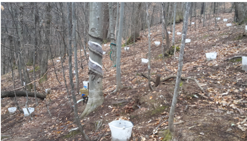
Figure 5.5: System of buckets for the total throughfall measurements. The buckets were installed and measures collected by the Department of Land, Environment, Agriculture and Forestry of University of Padua.
