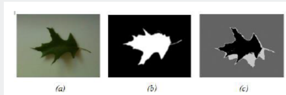
Fig.11. Segmentation results (a) the original image, (b) the segmentation result of the image by the modified EM algorithm, (c) the result of segmentation using Pseudo Zernike Moments of three channel images.
