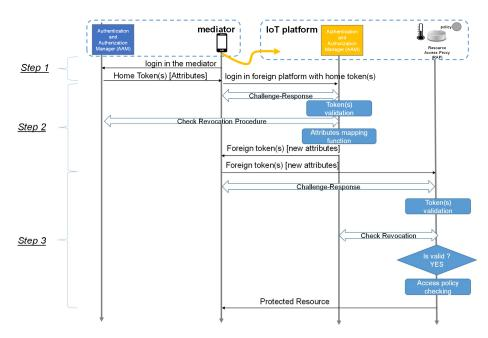
Fig. 2. An application registered in the mediator space would like to access resources in an IoT platform.
