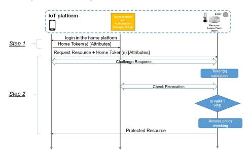
Fig. 3. An application registered in a given IoT platform wants to access resources produced within its home IoT platform.
