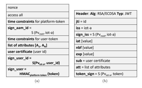
Fig. 5. Details of the content of (a) Macaroons and (b) JWT tokens for the designed architecture.
