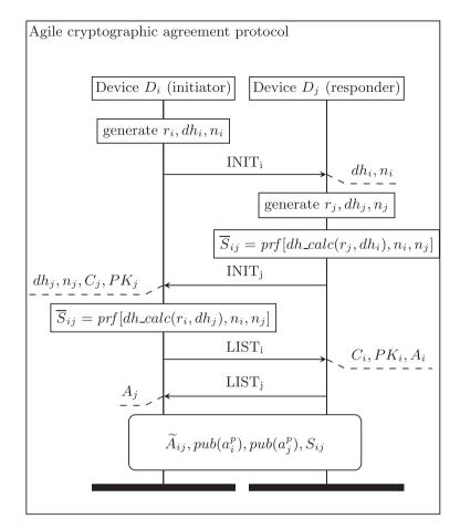
Figure 2. Agile cryptographic agreement protocol message exchange diagram.
