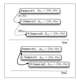
**Figure 10**. A scenario with a micro interval. First output is the left channel and second output is the right channel. First view is *temporal relations* and the second view is *dataflow relations*. It is better to represent separately both views of the score; otherwise, arrows will overlap.
