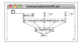
**Figure 7**. Pure Data patch representing the scenario in Figure 4. The Ntccrt plugin has only five outputs because the start of the second Karplus-Strong object (k2) is controlled directly from Faust. The internal clock of Ntccrt is controlled by a Pd *metronome* object with a period of 20 ms.
