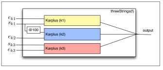
**Figure 6**. Block diagram representing the Faust process in charge of signal processing and the micro controls of the sound processors of the scenario. Signal processor @100 adds a delay of 100 samples to the signal  $s_{k1}$  (the start of the first string).
