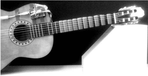
Figure 1. Gesture caption system based on capacitive sensors (mounted on the fretboard) and Arduino (mounted on the body).
