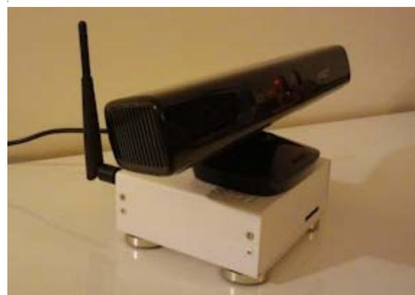
**Figure 6** - Embedded Kinect servers: (a) Panda board and the physical view of the prototype integrated with the MS Kinect for Windows device (b)
