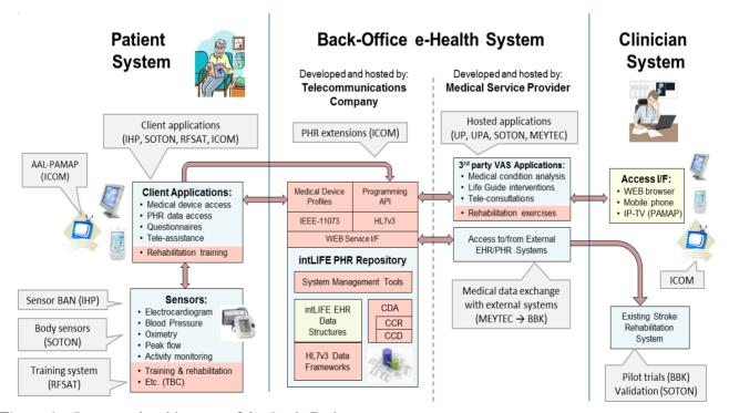
Figure 1 - Conceptual architecture of the StrokeBack system
