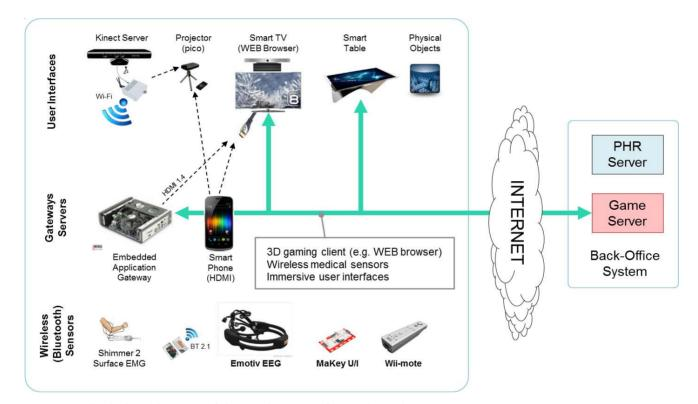
Figure 2 - Physical architecture of the gaming part of a StrokeBack system
