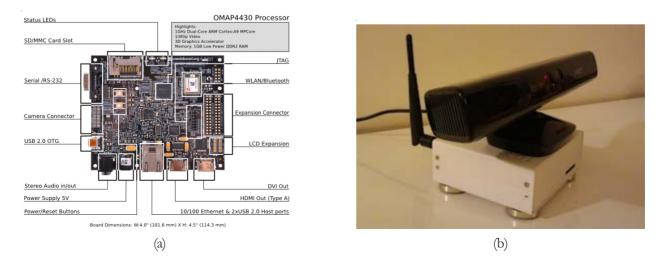
**Figure 6** - Embedded Kinect servers: (a) Panda board and the physical view of the prototype integrated with the MS Kinect for Windows device (b)
