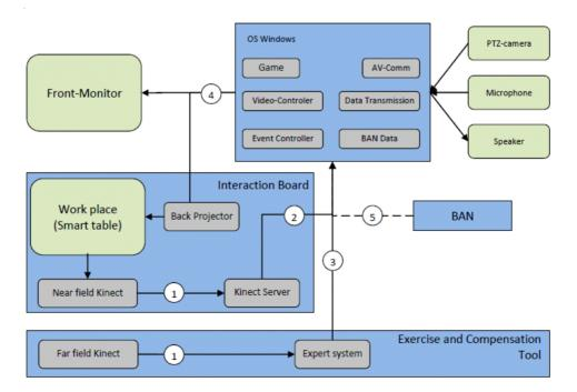
Figure 4 - Integration diagram of the overall home system of StrokeBack
