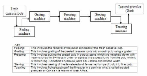
Figure 1: Flow-Chart of Gari Processing.
