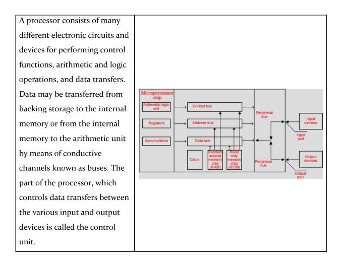
1. microprocessor chip, 2. registers, 3. accumulators, 4. control bus, 5. address bus, 6. data bus, 7. clock, 8. RAM, 9. ROM
