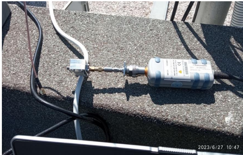
Figure 2-9: The USB power meter used for the alignment process
