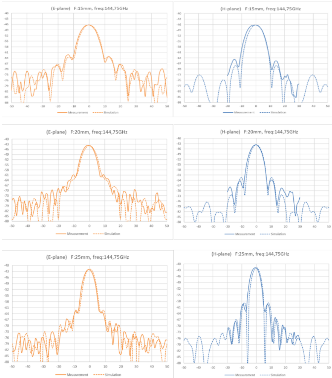
Figure 3-19: Radiation patterns E and H-planes of 0° tilted lenses for F=15mm, F=20mm and F=25mm
