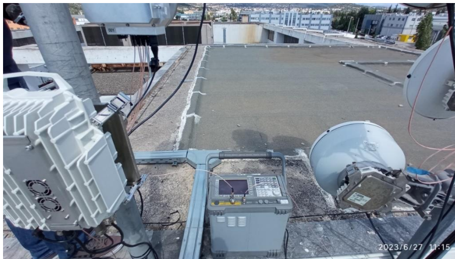
Figure 2-8: The spectrum analyzer used in the alignment process
