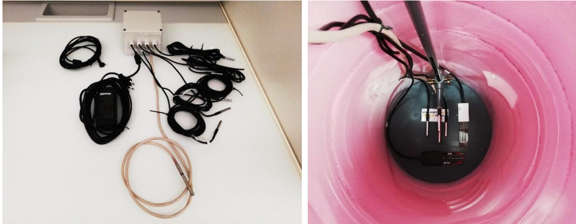
Figure 2. First version for MONitoring Temperatures in SEDiments (MONTSE) (left) and top view of the cylinder including all the sensors (right).
