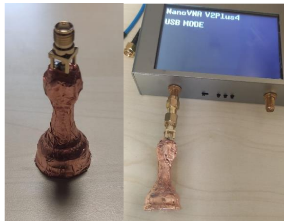
Figure 4. (a) SMA port soldered antenna (b) Nano VNA connection form
