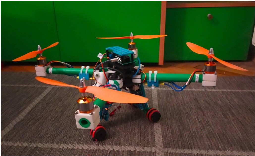
Figure 7 - Completed Drone - The drone houses all of the electronics shown in Figure 6, the frame of the drone is constructed out of polyvinyl chloride (PVC) pipes, and out of polylactic acid (PLA) three-dimensional (3D) printed plastic. Photo credit: Miloš Rašić.
