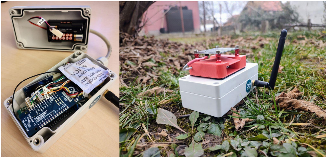
Figure 10 - Sensor Box - Sensor boxes are made to be completely weatherproof as well as waterproof, besides the Arduino they house sensors for measuring air pressure, temperature, humidity, and whether it is raining or not. Photo credit: Miloš Rašić.
