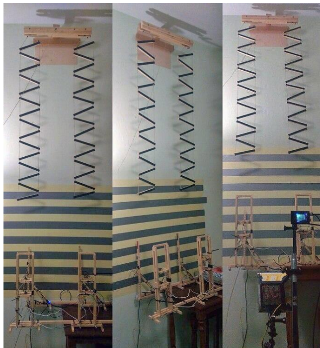
Figure 2 - Experimental Setup - The setup consisted of the quick release mechanism at the top, horizontal reference lines in the background, 120 frames per s (FPS) capable camera, and two sets of laser gates connected to an Arduino. Photo credit: Miloš Rašić.
