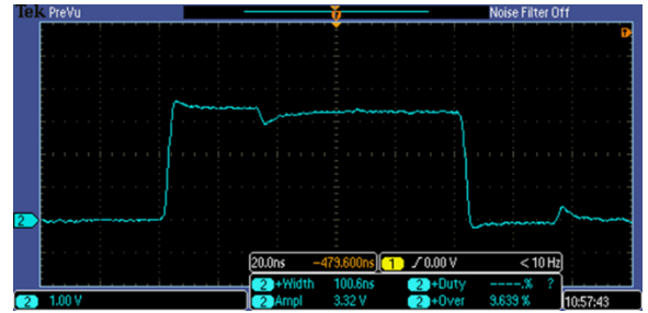
FIGURE 25. Injection pulse width = 100 ns
