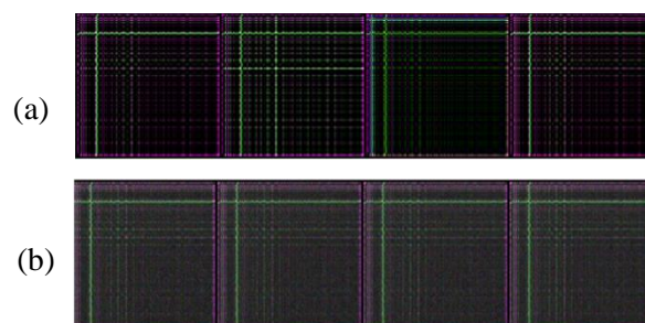
FIGURE 8. Original GASF signals (a) and synthesized by GAN (b)
