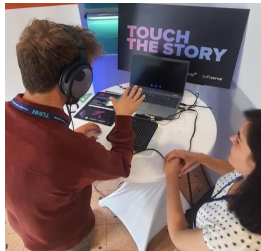
Figure 1: Demo setup showing a user interacting with the USX device while listening to the narrative via the headphones. The laptop is only used to make an initial selection of the narrative voice (male/female). The high table can be used for the user to rest their elbow, otherwise an armrest can be used instead.
