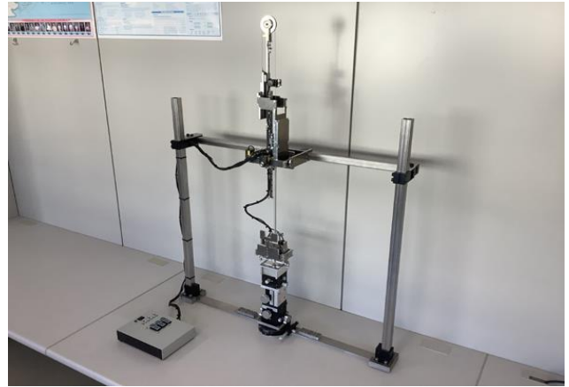
Fig. 2. The Contact Type Three-Dimensional Position-Measuring Instrument and the 6-Axis Stage
