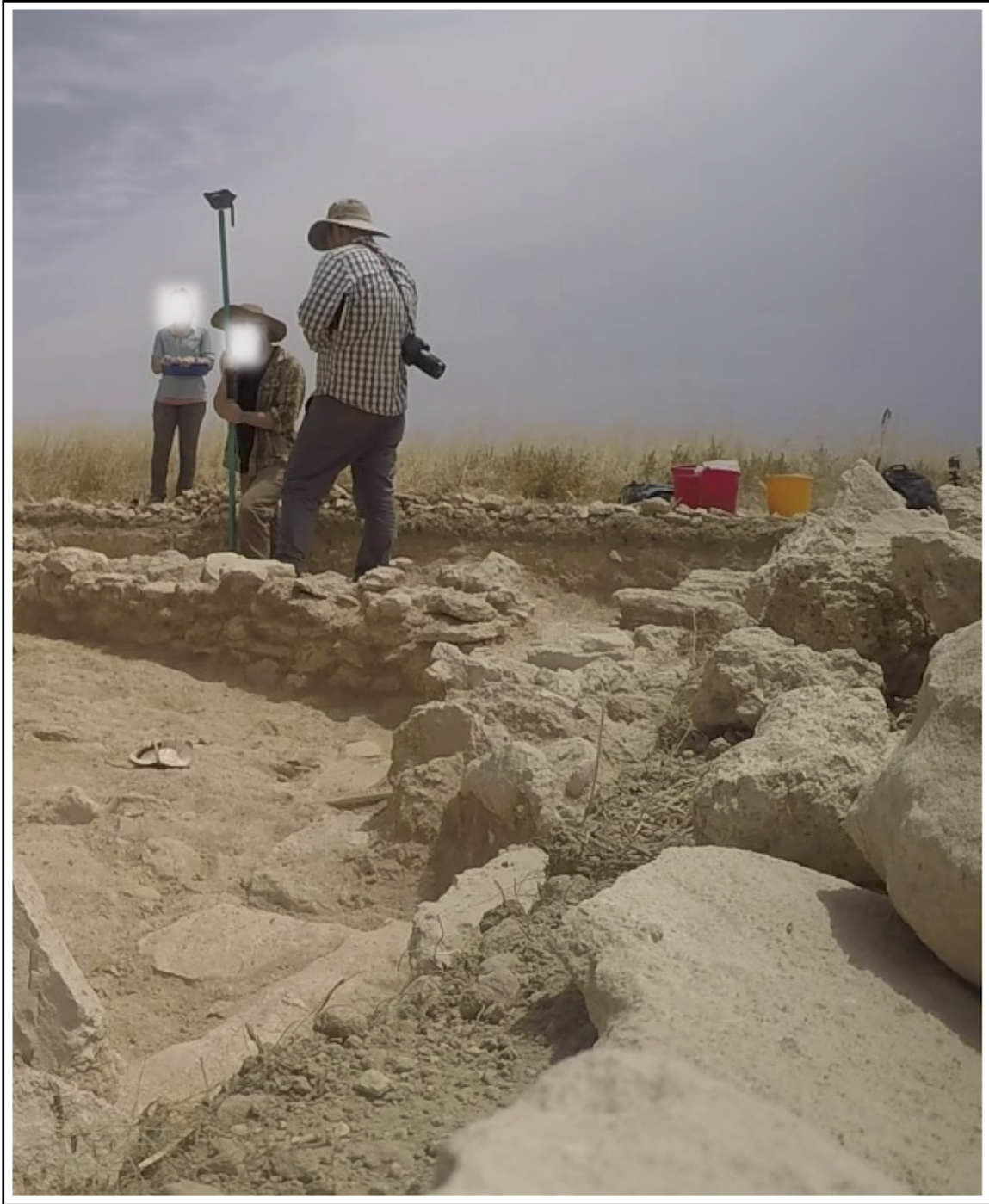
Figure 5.9: Recording DGPS points. The DGPS specialist records the geospatial point at the position where the trench assistant places the rover, while the trench supervisor oversees the process and identifies what needs to be recorded.
