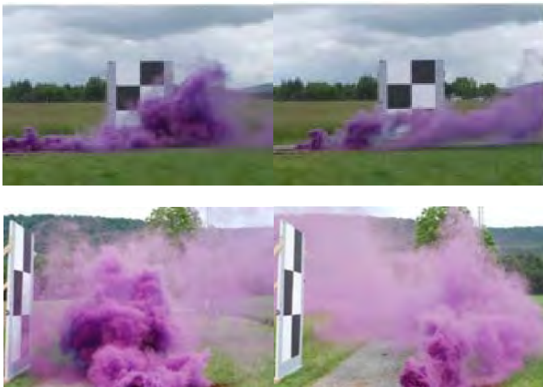
Figure 5-16 Emission of a passive substance 15 s (left) and 55 s (right) after the release. Side view (above) and view from behind (below) (from Long et al., 2010)
