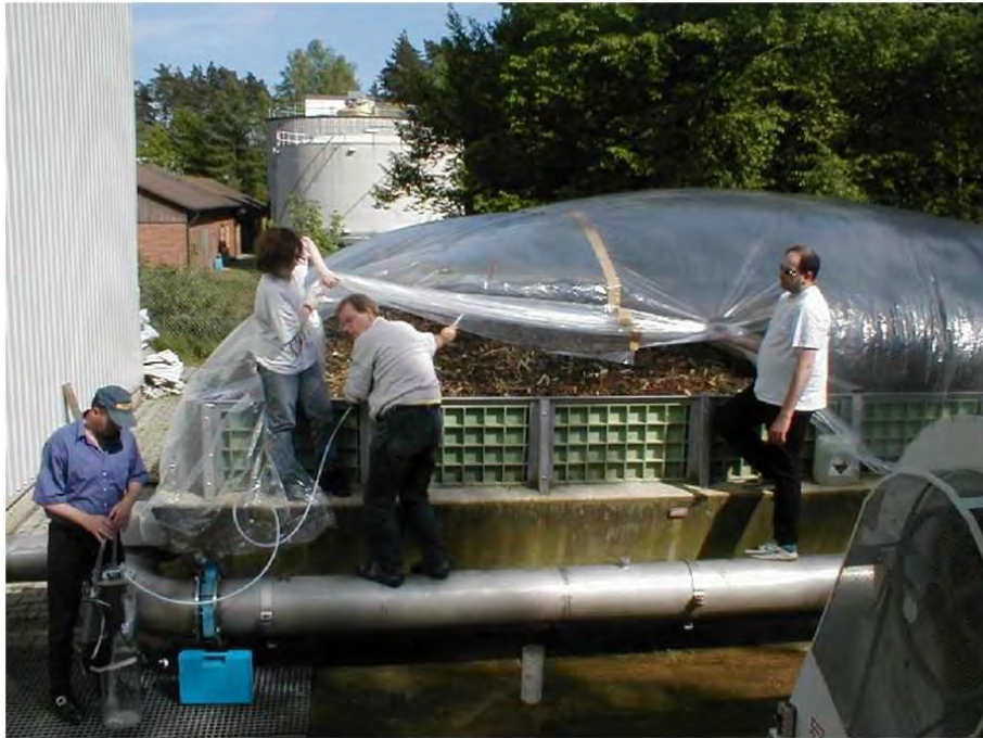
Figure 4-5 Complete coverage of an active area source (Courtesy of Mr. Franz-Bernd Frechen)
