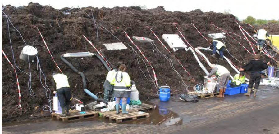
Figure 4-10 Sampling flux chambers and wind tunnels in a composting pile. (Courtesy of JM. Guillot)
