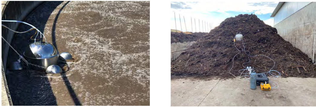
Figure 4-9 Flux chamber on a liquid source (left panel) and on a solid source (right panel)
