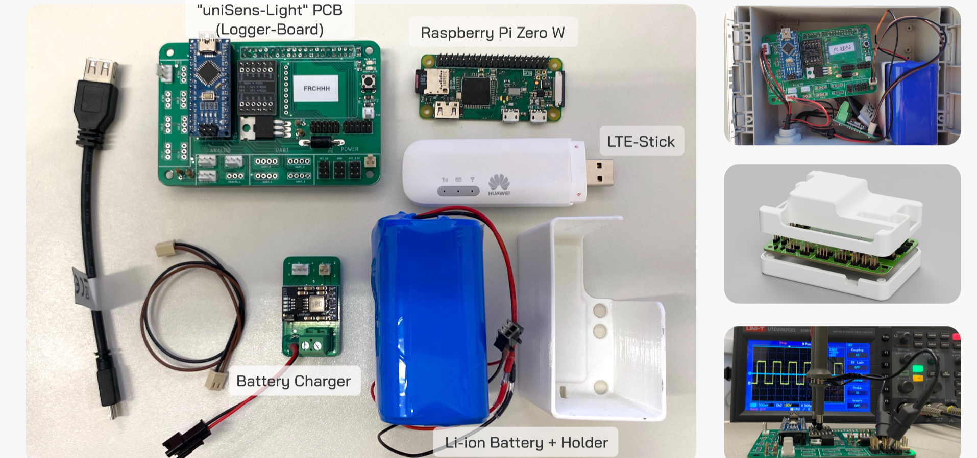
Fig. 3: "uniSens-Light" logger parts, field-deployed logger, logger-box rendering, PCB-test.
