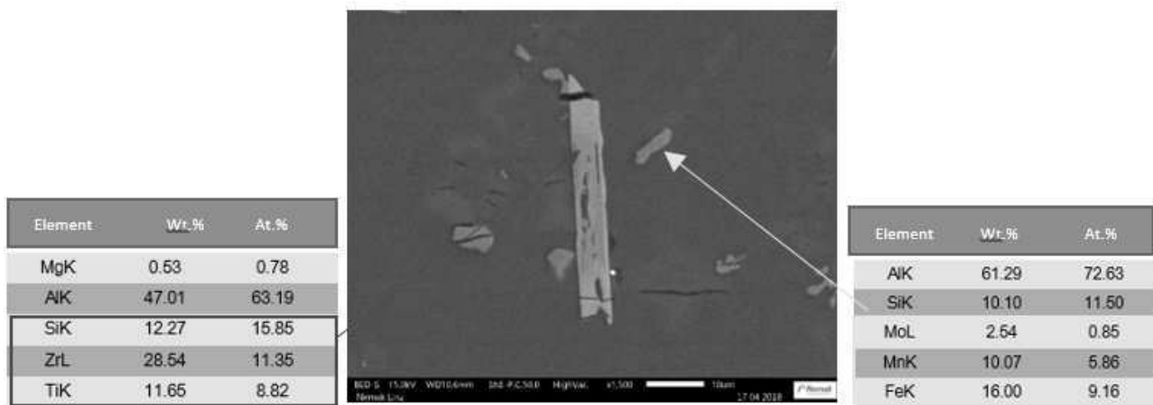
Fig. 10 EDX analysis of AlSi10MgCu alloy with 0.15 wt. % Mo and 0.15 wt. % Zr (exact amount of Mo – 0.1496 wt. %, Zr – 0.128 wt. %), without heat treatment - sample C, SEM
