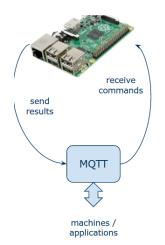
Fig. 2. Mqtt-based messaging communication
