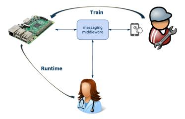
Fig. 4. MQTT-based calibration procedure
