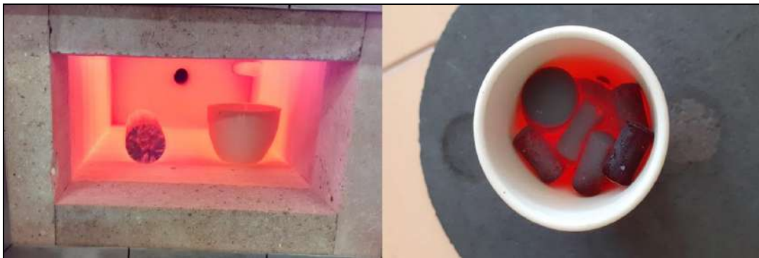
Figure 1 Heat treatment of steel samples in an electric resistance furnace
