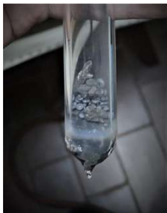
Figure 2 Elementary components loaded into cleaned quartz tubes
