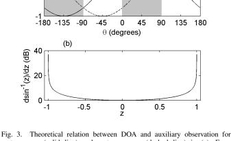
Fig. 3. Theoretical relation between DOA and auxiliary observation for system  $\mathbf{x}, \mathbf{y}$  (solid line) and system  $-\mathbf{x}, \mathbf{y}$  (dashed line) in (a). Error sensitivity of any of the two estimators as a function of the actual value of the auxiliary observation is shown in logarithmic scale in (b).
