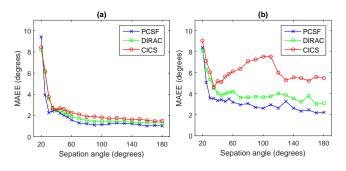
Fig. 8. MAEE for two speakers inside a simulated environment as a function of source separation angle. Results are shown at 10 dB SNR for  $RT_{60} = 200$  ms in (a),  $RT_{60} = 400$  ms in (b).
