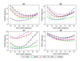
Fig. 6. MAEE for each technique as a function of the length of the Blackman sequence used for constructing the atoms for MP. Results are shown for three speakers in a simulated environment of  $RT_{60} = 400$  ms and SNR=30 dB of isotropic noise in (a),  $RT_{60} = 200$  ms and SNR=5 dB of isotropic noise in (b),  $RT_{60} = 200$  ms and SNR=5 dB of common mode noise in (c) and  $RT_{60} = 200$  ms and SNR=5 dB of spatially white noise in (d).
