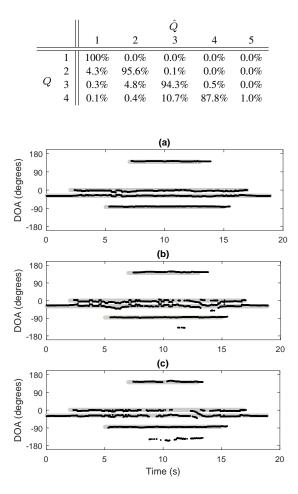
Fig. 10. Estimated DOA of four static speakers in a real environment using PCSF in (a), DIRAC in (b) and CICS in (c).
