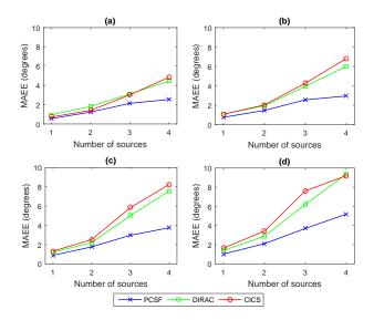
Fig. 7. MAEE for each technique at 30 dB SNR of spherical isotropic noise as a function of the number of speakers for  $RT_{60} = 200 \text{ ms in (a)}$ ,  $RT_{60} = 300 \text{ ms in (b)}$ ,  $RT_{60} = 400 \text{ ms in (c)}$  and  $RT_{60} = 500 \text{ ms in (d)}$
