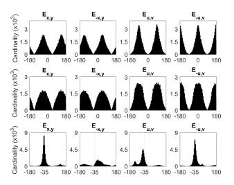
Fig. 4. Histogram with the candidate DOAs as obtained from for each one of the four estimators rising from the case of the square array for spherical isotropic noise (top row), spatially white noise (middle row) and single acoustic source at  $-35^{\circ}$  inside a reverberant room (bottom row).
