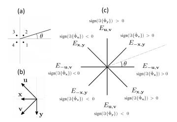
Fig. 2. Square sensor configuration in (a) and corresponding vectors in (b). Maximum Robustness Axes and corresponding disambiguation criteria for each one of the four estimators rising from the case of a square array in (c)
