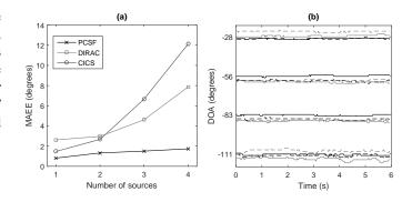
Fig. 9. Sound source localization in the real environment. MAEE as a function of the number of speakers in (a) and estimated DOA as a function of time for four different single active speaker locations for PCSF (blue), DIRAC (green), CICS (red) and CHB (black) in (b). The true DOAs are at -28, -56, -83 and -111 degrees.
