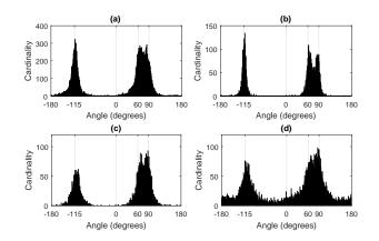
Fig. 5. Histogram with the DOAs obtained from PCSF after candidate DOA fusion in (a) and after local DOA fusion in (b). Histogram obtained for the same conditions using DIRAC is shown in (c) and using CICS in (d). Results are shown for a simulated reverberant environment of  $RT_{60} = 300$  ms with three simultaneous sources at -115, 60 and 90 degrees.
