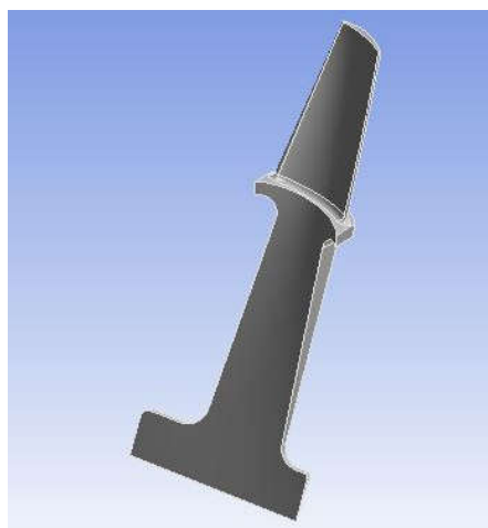
Fig 2. Sector Model of Turbine Blisk
