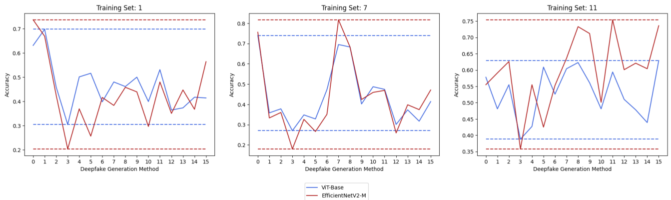
Figure 2: Line plots representing the accuracy values obtained by ViT-Base (blue) and EfficientnetV2-M (red) on the test set, trained on training sets consisting of real images and from left to right on images generated with the FaceShifter, Talking Head Video and StyleGAN2 methodology respectively. Observing the space between horizontal lines it is possible to notice how the variance of the Vision Transformer is lower than that of the CNN counterpart obtaining closer accuracies on different and also unseen methods. On the horizontal axis the 0 represent the real images and number from 1-15 the images generated with different generation methods.
