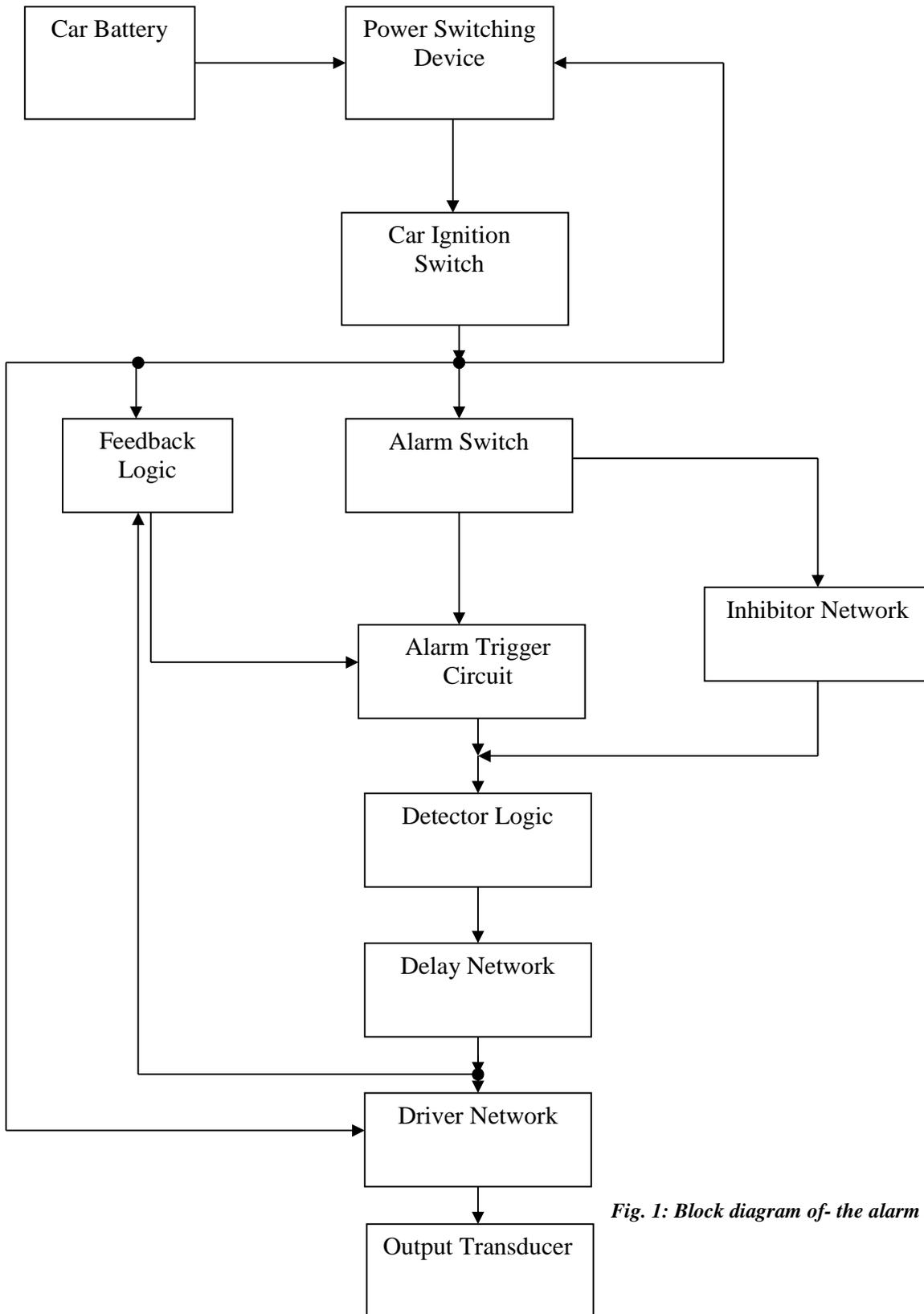
Fig. 1: Block diagram of- the alarm system
