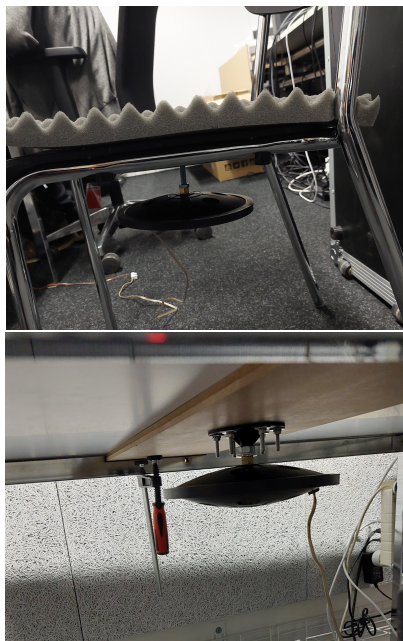
Figure 1. Transducers under the chair (top) and under the tabletop (bottom).
