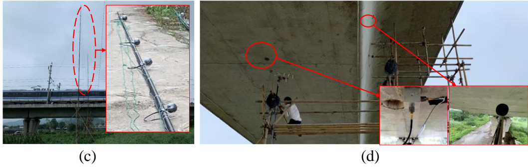
Figure 3. (a) Suburban train (b) Data acquisition system (c) Setup of one microphone array, and (d) Setup of microphone and accelerometer under the bridge.
