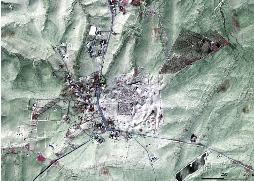
277 Figure 7 - Pansharpened product of the datafusion technique by panchromatic and multispectral data 278 of Pléiades Neo-04 image.
